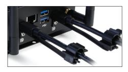
The cable tie slides into the cable tie base while the connector is being plugged into the device.
