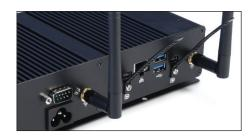
The cable lock system is made from two parts. The cable tie base that is placed around the connecting cable and a cable tie that is screwed onto the device.
